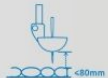
压脚可根据物料厚度调节 Presser foot can be adjusted according to different thickness
